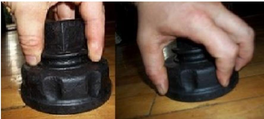
Comparison of Nozzle Cover: Gripping Lip (left) and Gripping Base (right)
